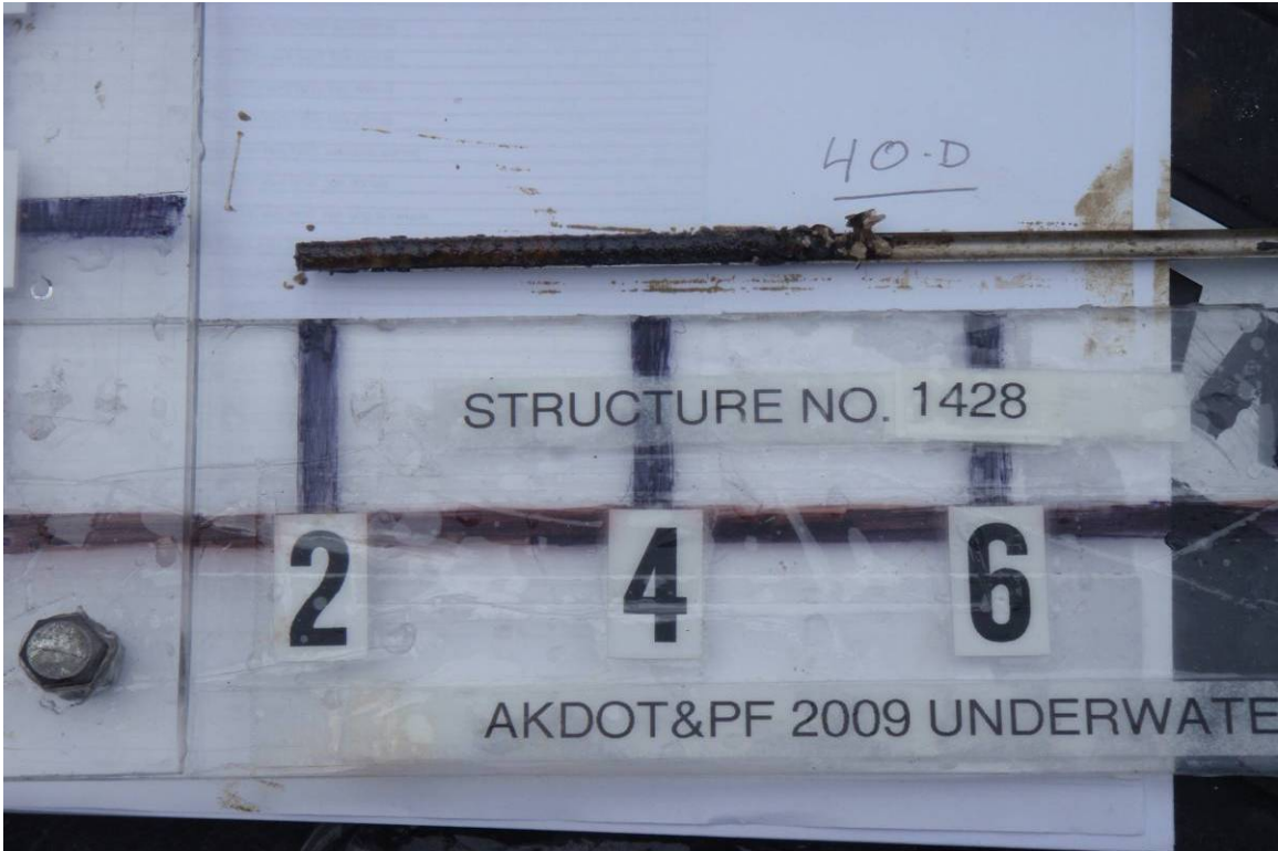
Photograph 5 – Typical Timber Core
