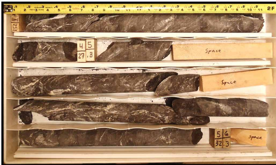
RM12-04, Box 2, 25.1 to 32.3 feet, Dry. Core box highlighting the higher rock quality and visible carbonate veins observed within the phyllitic graywacke unit
