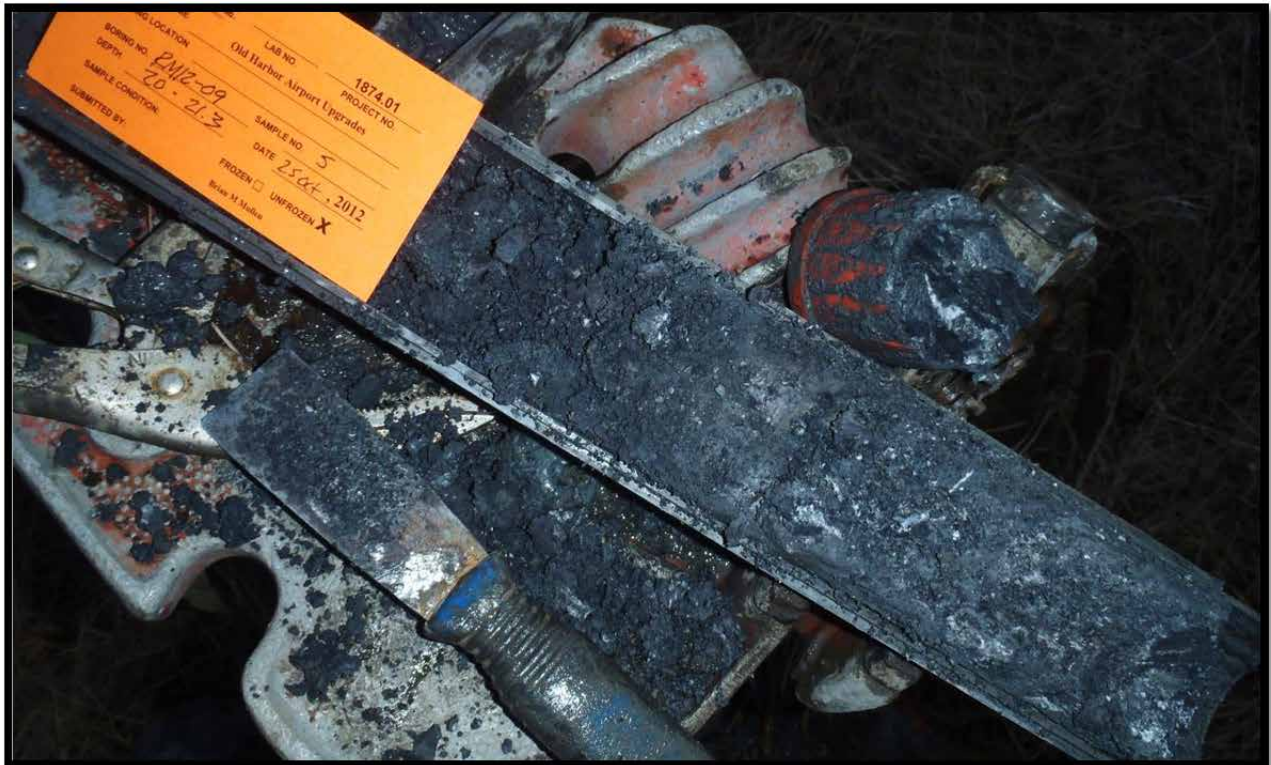
Test Boring RM12-09, Sample 5, 20.0 to 21.3 feet, Sample within the weathered bedrock unit
