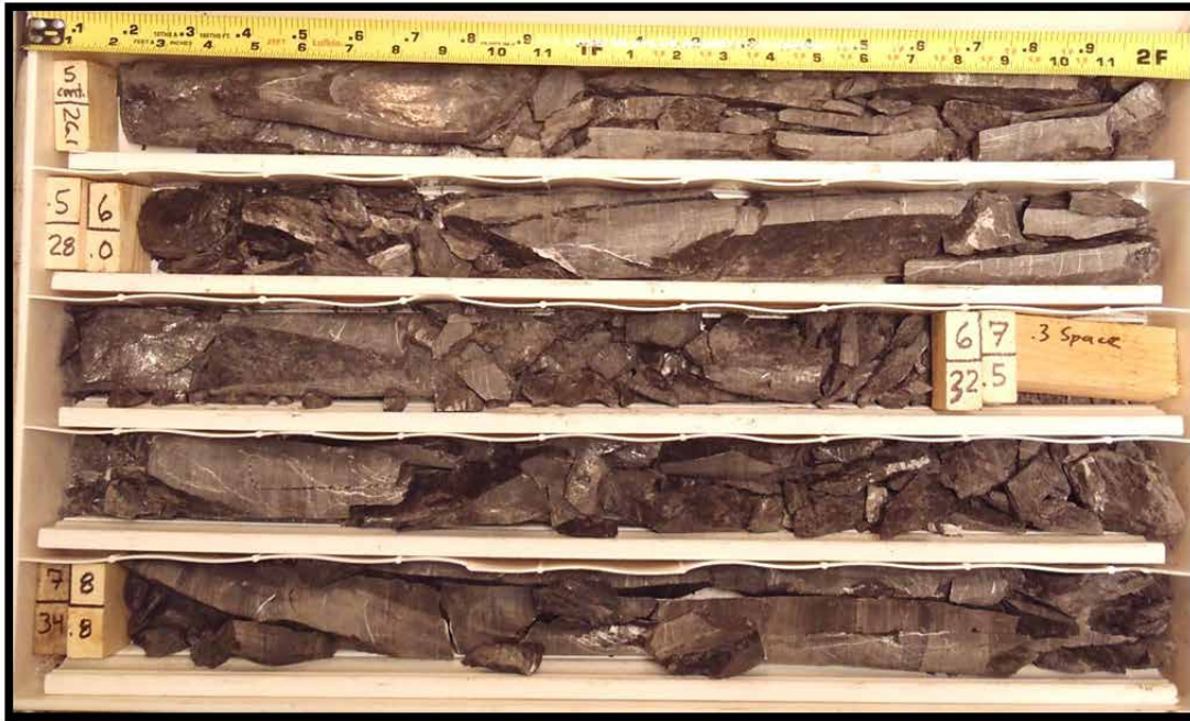
RM12-03, Box 2, 26.1 to 37.2 feet, Dry. Core box highlighting the highly fractured recovery and vertical trending foliation observed within many zones of the phyllite unit
