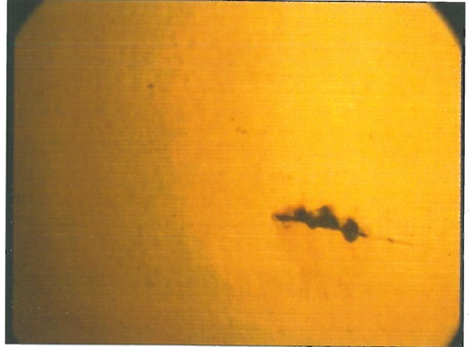
Large cracked blister on mid shell coating (Time 17:33)
