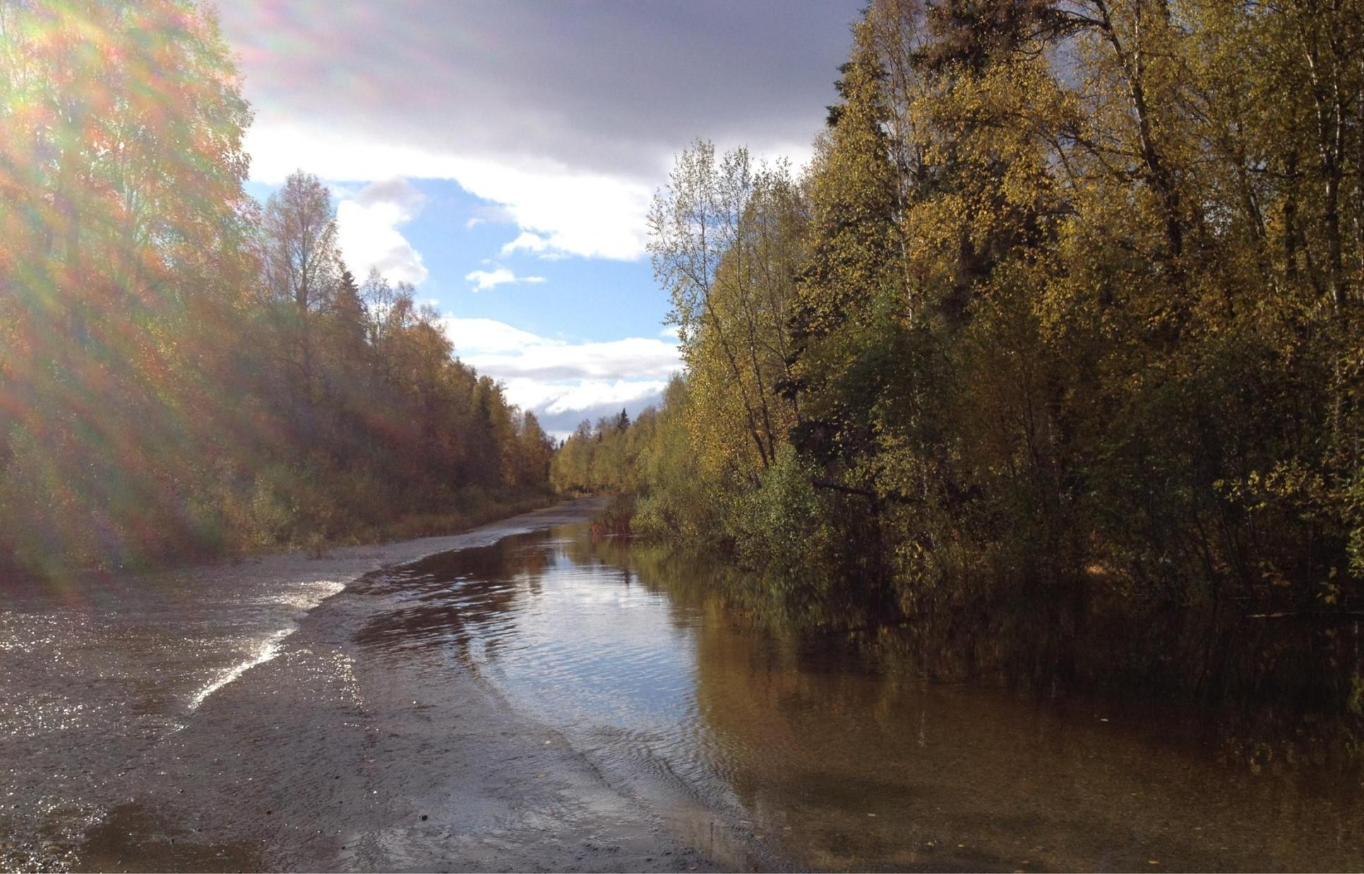
September 2012. Oilwell Road becomes impassible frequently because of poor drainage and improper road elevation. Frequent damage to the road costs the Mat-Su Borough thousands of dollars in repairs annually and cuts off over 400 local residents from food and emergency services.
