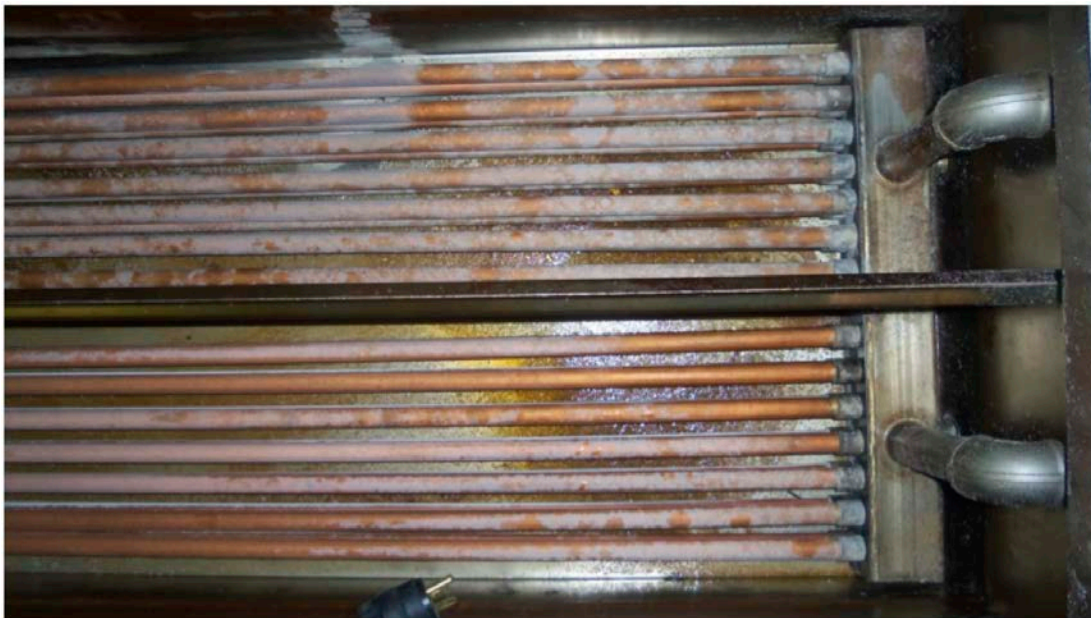
Figure STEAM 25. Torre's radiator design that is used to pipe steam through sap.
