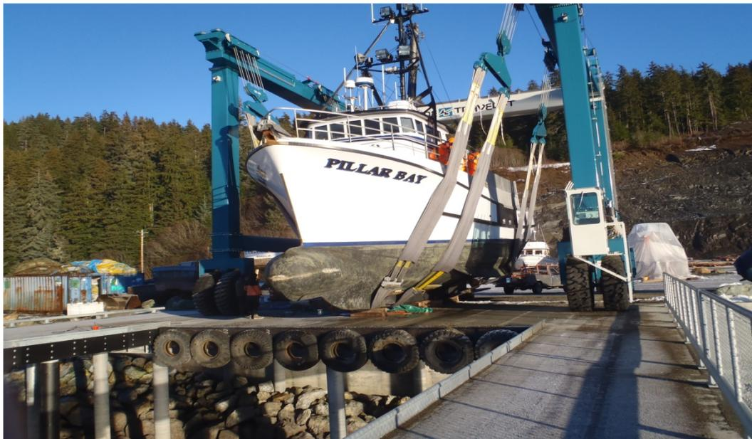
This 190-ton seiner was lifted out in December 2010 for limited maintenance and repairs. Until Phase III is completed, only limited services can be performed on boats as the treatment of wastewater and stormwater via the washdown facility is essential for compliance with state and federal environmental standards.
