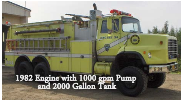
1985 Engine with 1000GPM Pump and 2000 Gallon Tank
